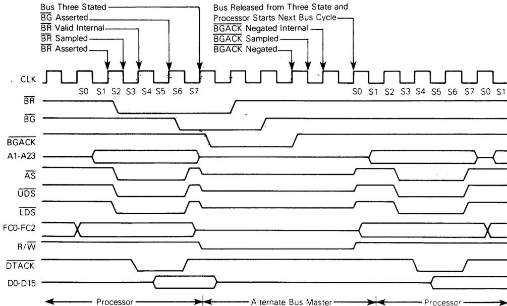
Figure 4-15. Bus Arbitration Timing Diagram — Processor Active
