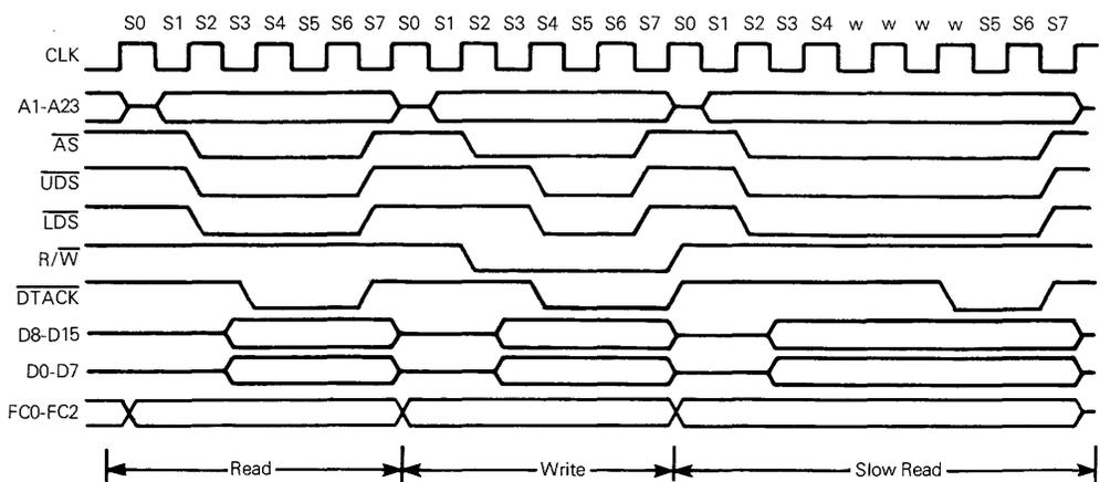
Figure 4-4. Read and Write Cycle Timing Diagram
