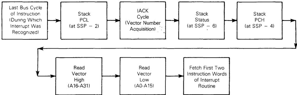
NOTE: SSP refers to the value of the supervisor stack pointer before the interrupt occurs.
