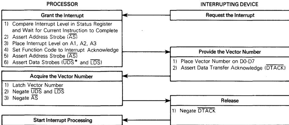
\* Although a vector number is one byte, both data strobes are asserted due to the microcode used for exception processing. The processor does not recognize anything on data lines D8 through D15 at this time.
