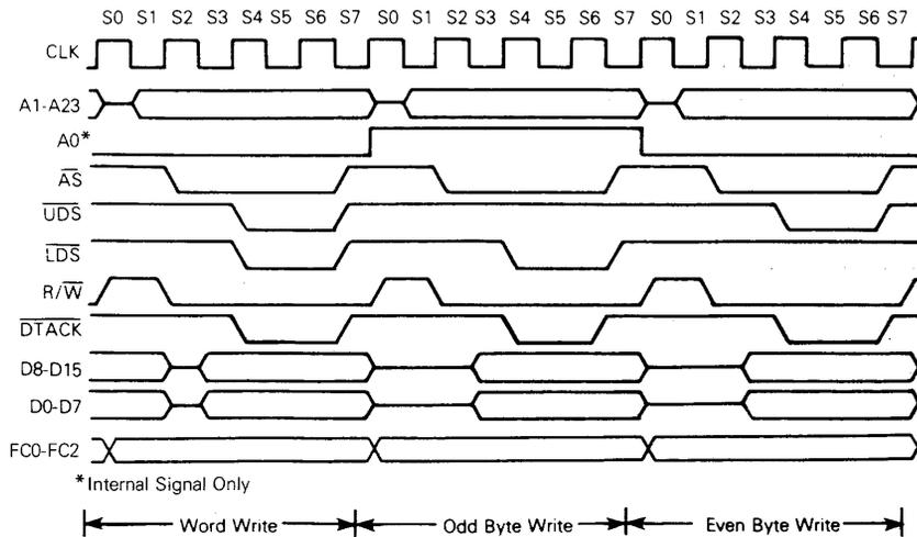
Figure 4-8. Word and Byte Write Cycle Timing Diagram
