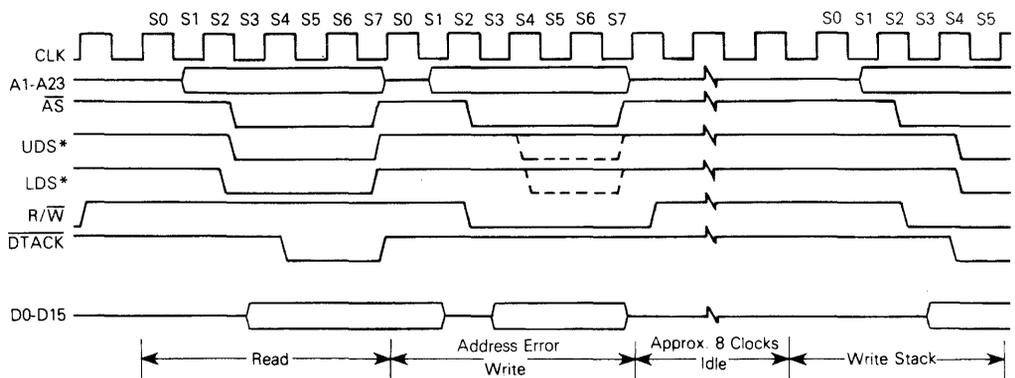
\* $\overline{UDS}$  and  $\overline{LDS}$  are asserted on mask sets R9M, BF4, T6E, DL6, CC1, and GN7.
