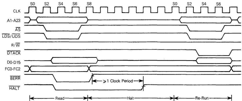
Figure 4-19. Re-Run Bus Cycle Timing Diagram
