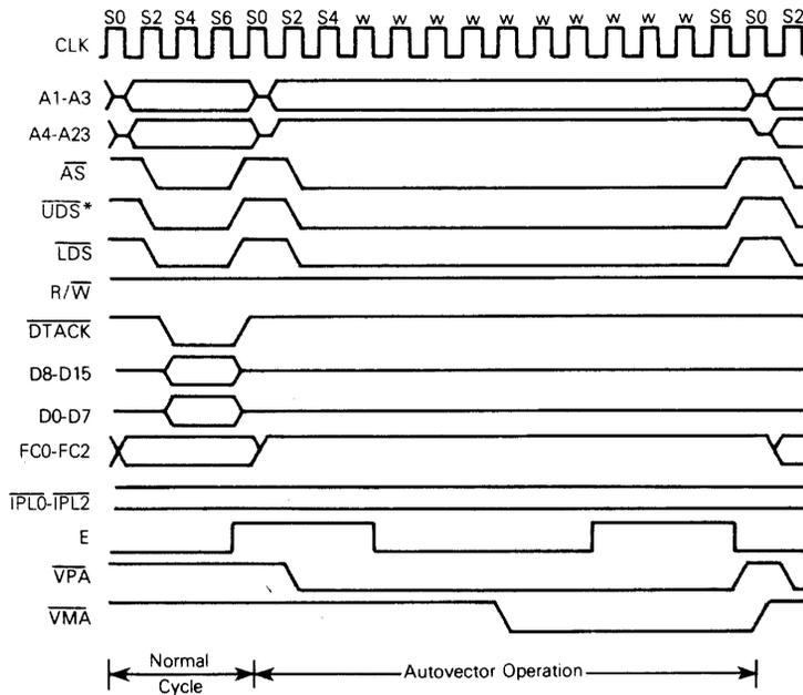
\* Although a vector number is one byte, both data strobes are asserted due to the microcode used for exception processing. The processor does not recognize anything on data lines D8 through D15 at this time.
