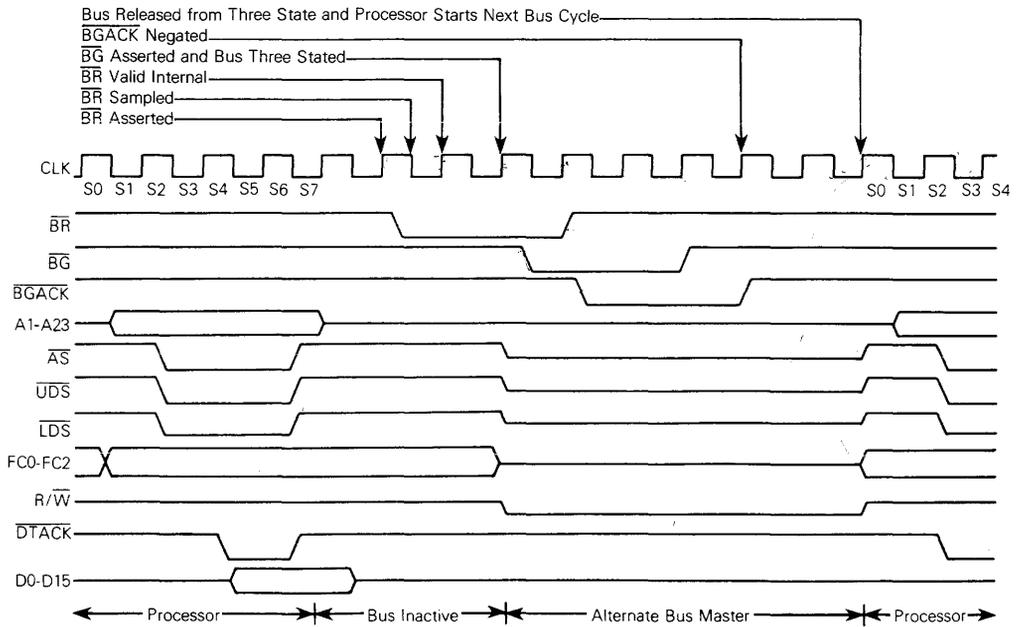
Figure 4-16. Bus Arbitration Timing Diagram – Bus Inactive
