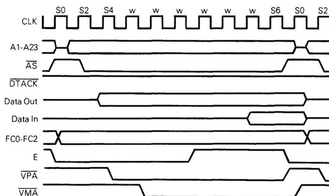
Figure 6-2. MC68000 to M6800 Peripheral Timing — Best Case
