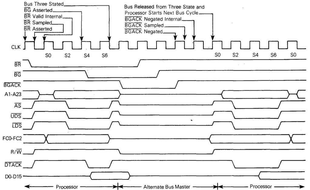
Figure 4-17. Bus Arbitration Timing Diagram – Special Case
