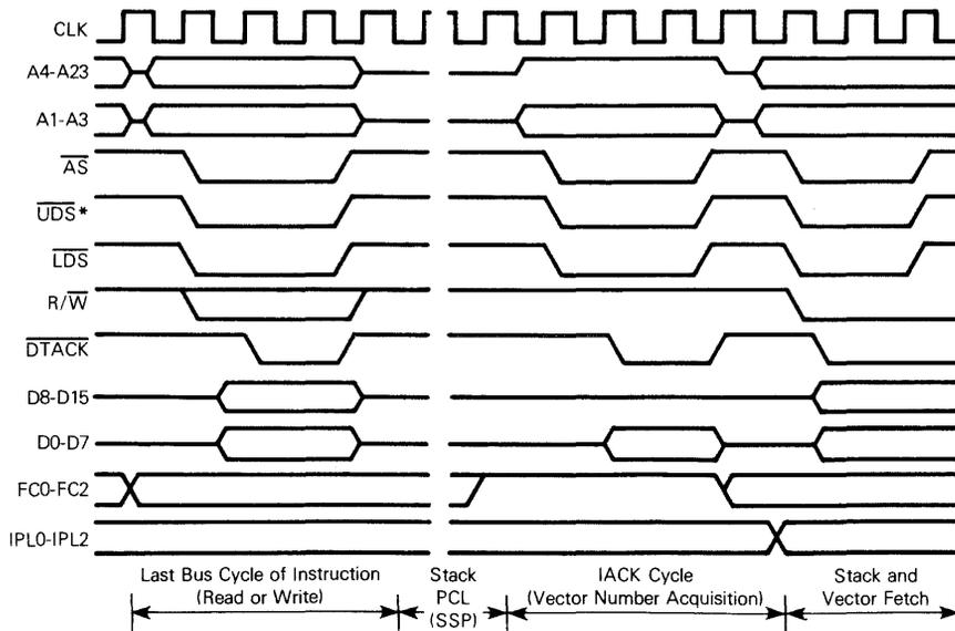
\* Although a vector number is one byte, both data strobes are asserted due to the microcode used for exception processing. The processor does not recognize anything on data lines D8 through D15 at this time.
