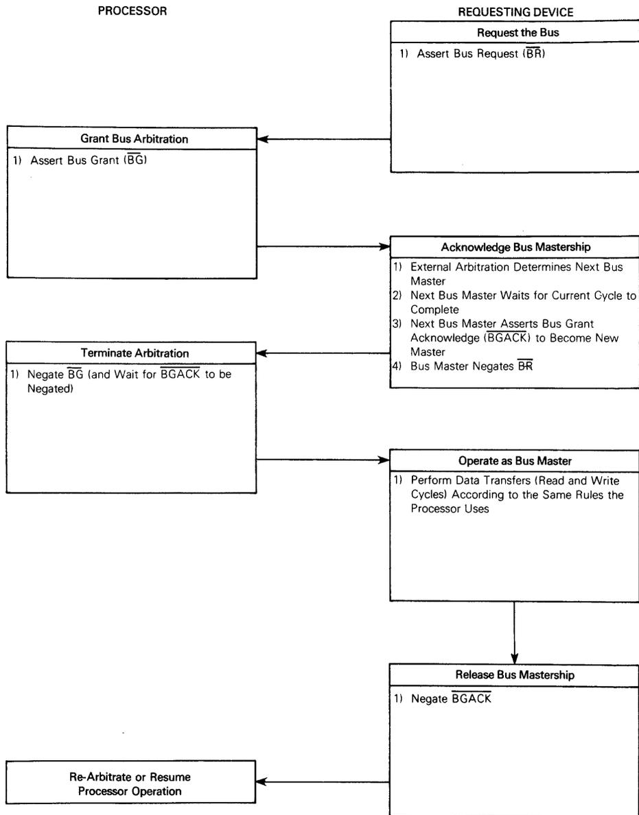
Figure 4-11. Bus Arbitration Cycle Flowchart
