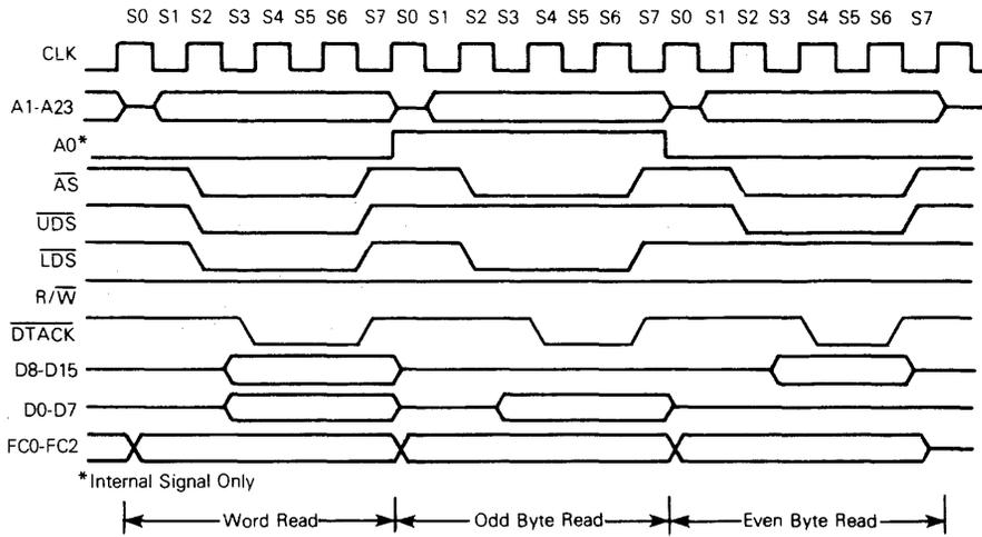
Figure 4-5. Word and Byte Read Cycle Timing Diagram
