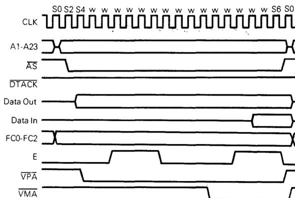
Figure 6-3. MC68000 to M6800 Peripheral Timing — Worst Case
