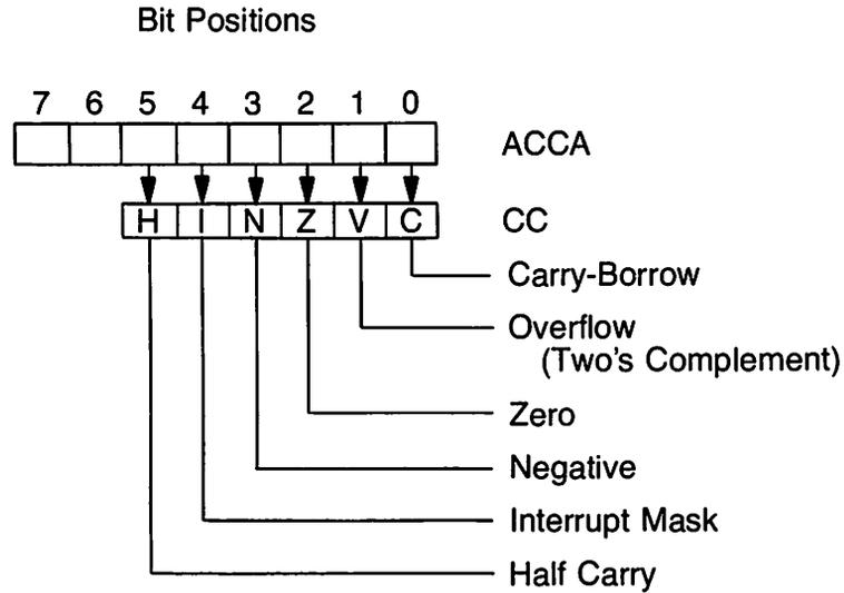
**Description:** Transfers the contents of bit positions 0 thru 5 of accumulator A to the corresponding bit positions of the processor condition codes register. The contents of accumulator A remain unchanged.
