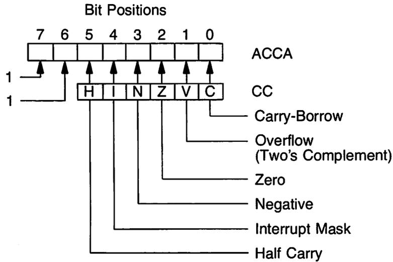
Description: Transfers the contents of the processor condition codes register to corresponding bit positions 0 thru 5 of accumulator A. Bit positions 6 and 7 of accumulator A are set (i.e. go to the "1" state). The processor condition codes register remains unchanged.
