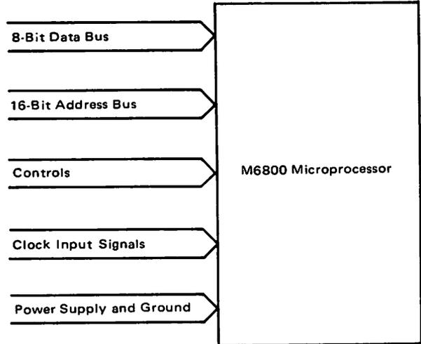
FIGURE 2-3. M6800 Microprocessor – Inputs and Outputs
